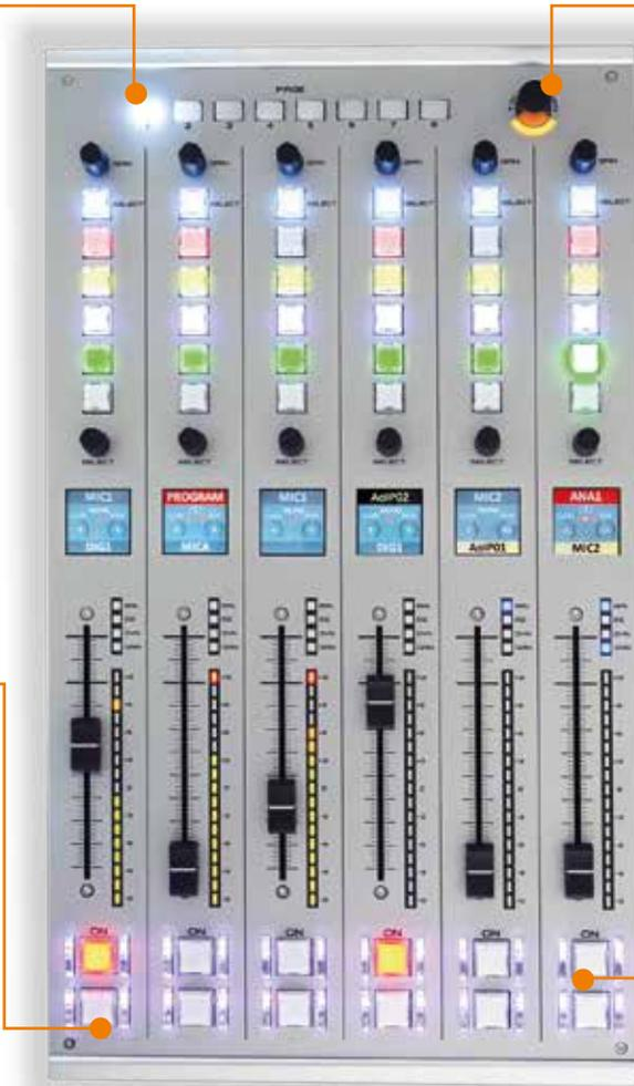
Next to the page swap keys, there is a touch & turn rotary encoder to perform precise adjustments on the touch screen.
