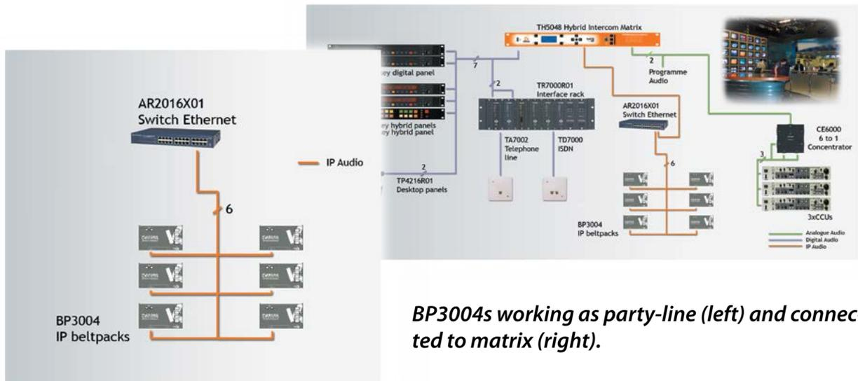
*BP3004s working as party-line (left) and connected to matrix (right).*
