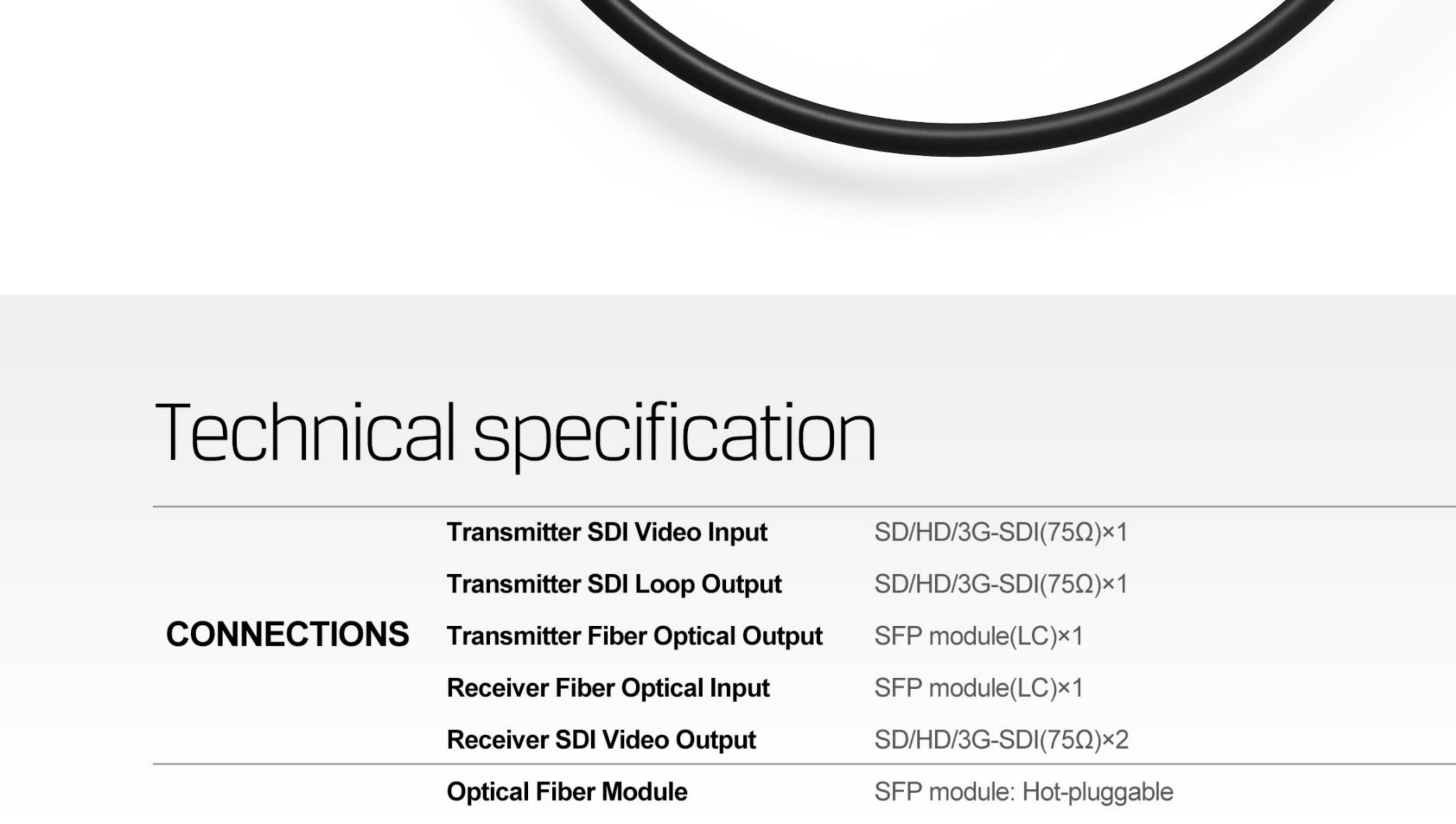
Equalized on the SDI input and reclocking on the SDI outputs to maximize performance up to 120m for 3G and 140m for HD-SDI. It ensures transmission quality and effect of eye diagram, and fully compatible with 3G level A & level B formats.
